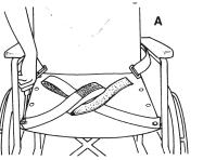
**3.** Behind the wheelchair, remove the screws second from the bottom on the left and right sides of the backrest. Insert the screws through the grommets on the **belt sections fitted with d-rings.** Reinsert the screws into the holes in the wheelchair backrest. Tighten screws. (See Illustration B.)
